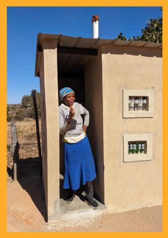
a long drop toilet (loo) built using both ecobricks and regular blocks.
